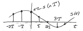
Output of a sampler is sometimes called sampled analog.
